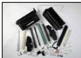
Traditional laser printer cartridge containing many components, comprising various materials
